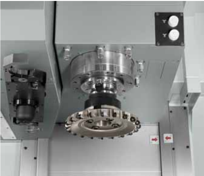
Fig 2. No. 50 Taper Spindle (with 240 mm face mill)
